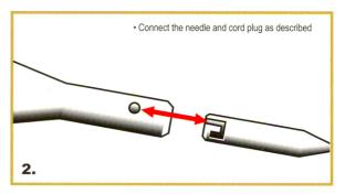
**Step 2:** The open recess in the cord plug and the inset point at the end of the needle must line up exactly (picture 2) for the needle to lock in easily.
