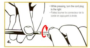
**Step 4:** While pressing, turn the cord plug roughly  $^{1}/_{16}$  of a turn to the right until it locks into position, (picture 4). So cord and needle fit together perfectly.
