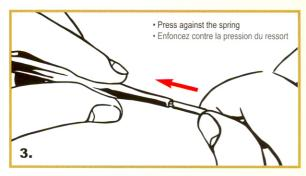
**Step 3:** Insert the cord plug (picture 3)  $^{1}/_{8}$  of depth into the needle thus compressing the spring in the needle; this may require a bit more strength the first time, you are using your clicks.
